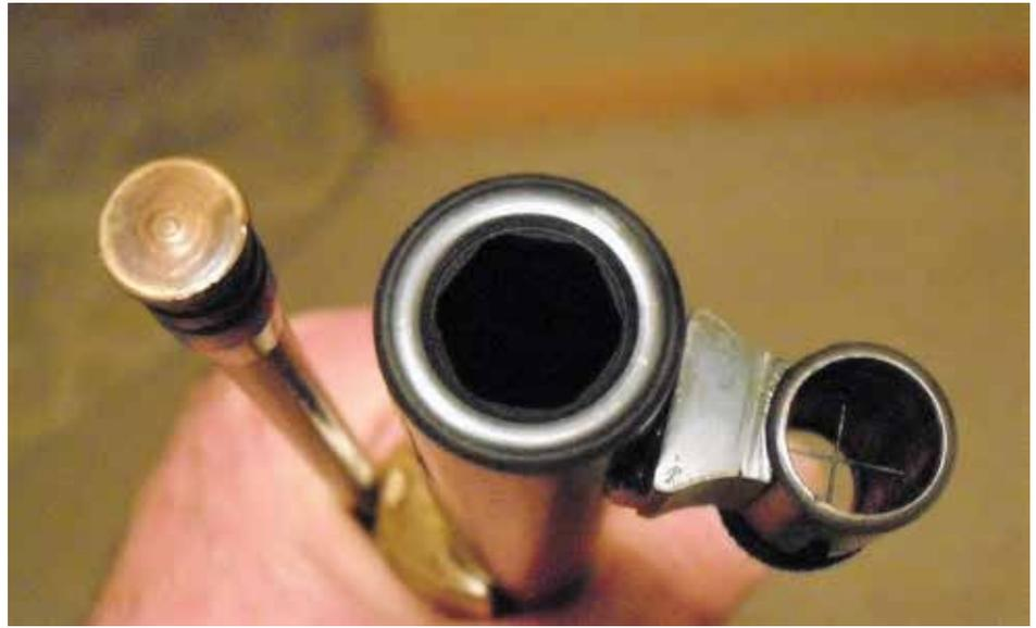
*Muzzle of a Whitworth rifle showing the hexagonal bore.*
